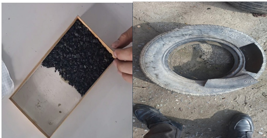
Figure 1. Tires from which samples were taken for the laboratory process of obtaining a composite material from car tires.
