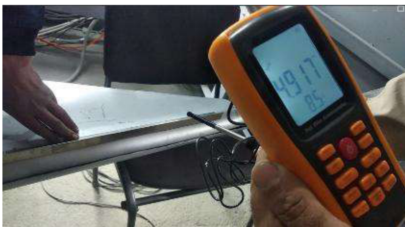
4-rasm. Havo pudash tizimi tirqish 5 mm arragacha masofa 65 mm
