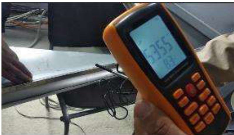
3-rasm. Havo pudash tizimi tirqish 5 mm arragacha masofa 45 mm
