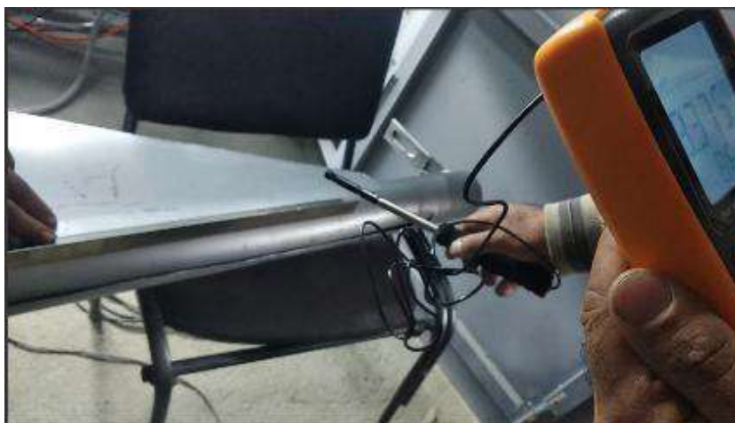
5-rasm. Havo pudash tizimi tirqish 5 mm arragacha masofa 85 mm
